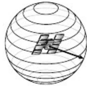
First measurement puts us somewhere on this sphere.
